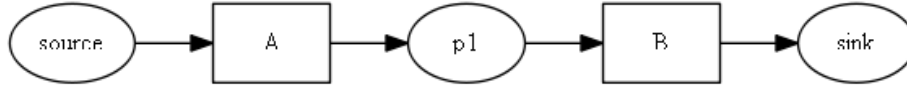
Fig. 2: Example sequential Petri net. From the initial state (source), the transitions A and B could be used to reach the final state (sink).
